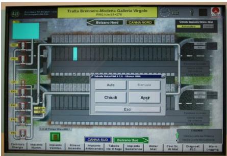
SCADA Control System
